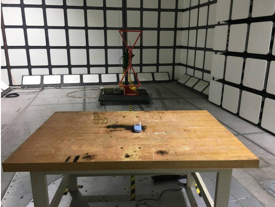
Radiated Emissions View (Below 1 GHz)
